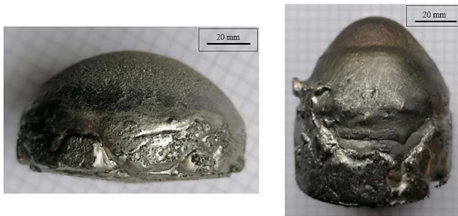
Figure 3. Experimental results with the injection of inert gas: solidified sample with the volume of 65 cm 3 (left) and 130 cm 3 (right). Free surface deformation is still visible as result of the rapid solidification of the cast.
