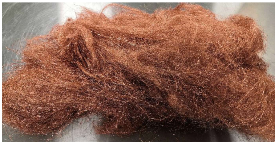
Figure 2. Copper yarn with continuous 20\mu thick filament.
