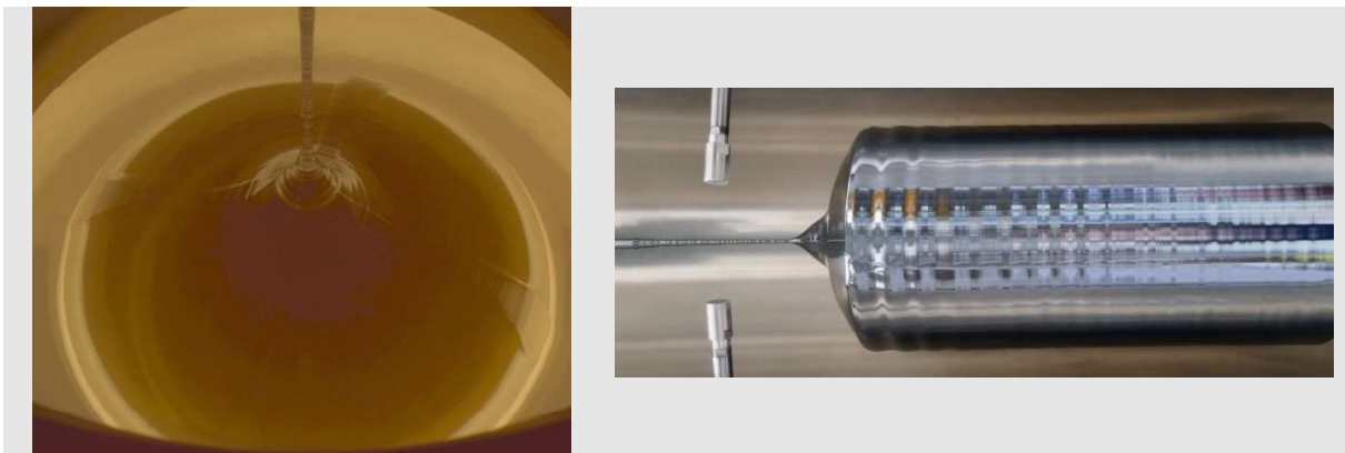
Figure 1: Growth of a 300 mm Crystal at the Fraunhofer CSP. Shoulder growth (left) and 300 mm crystal (right)
