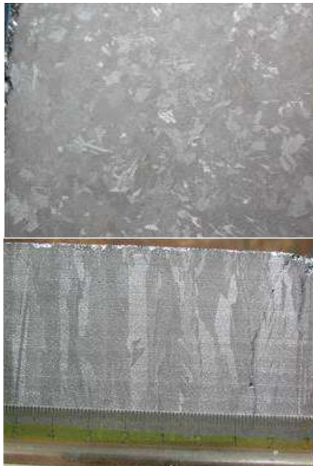
Figure 9. Photo of a cross section and of a side of a brick cut from the ingot.
