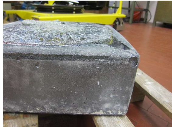
Figure 8. The ingot casted and solidified at LEP. The upper layer of the ingot is mostly silicon carbide.
